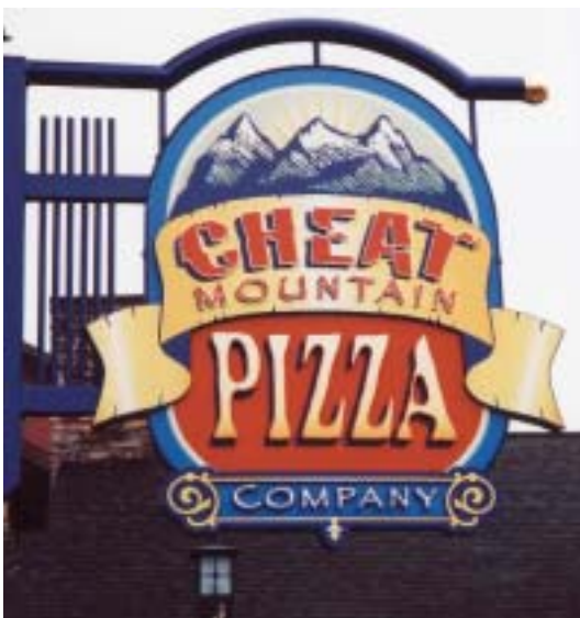
Graphic and Cheat are vinyl, printed on the Gerber Edge®; remaining copy is vinyl. Panel is PVC with 1/2-in. PVC ribbon, finished with Matthews. Sign is 36 by 36 in. overall, and is mounted in a wrought iron bracket.
