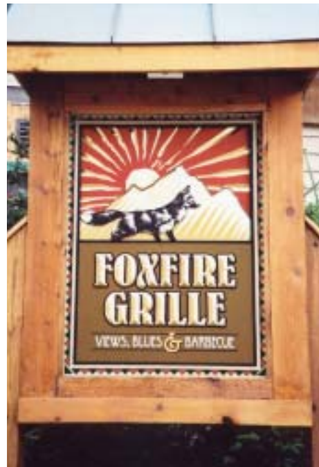
Main copy is prismatic, routed from Sign-Foam high-density urethane board and finished with 23k gold leaf; secondary copy is vinyl. Fox and mountains are vinyl, printed on the Gerber Edge® and mounted on PVC cutouts. Border is vinyl film. Sun's rays are carved and gilded. This 32-by-42-in. double-faced sign has five layers of substrate and has cedar trim with a copper roof.
