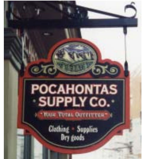
Vinyl lettering and graphics on 24-by-26-in. panel of double-faced 3/4-in. overlaid plywood. Oval and scrolls are routed 1/2-in. PVC, painted with Matthews Polyurethane. Graphic in oval was printed on the Gerber Edge®. Bracket is wrought iron.
