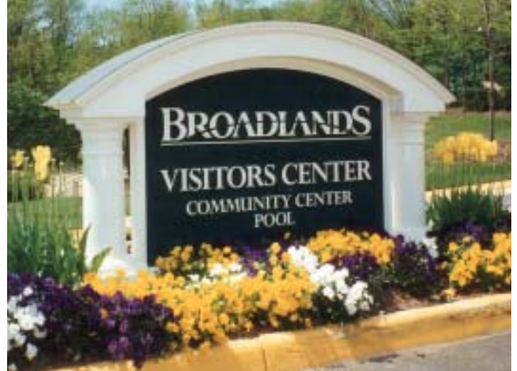
Sign-Foam [Sign Arts Products, 800-338-4030, www.signfoam.com ] high-density urethane board lettering finished with acrylic latex paint on 44-by-64-in. high-density urethane board panel over an overlaid plywood structure. The roof is copper over a PVC cap; columns are PVC. Sign is 16 in. thick.
