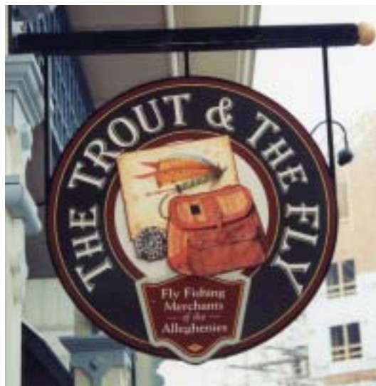
Lettering and graphic are vinyl, printed on the Gerber Edge®. The 28-in. diameter panel is 3/4-in. plywood laminated on both sides with PVC, painted with 1Shot enamel. Bracket is wrought iron.
