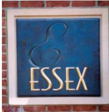
Lettering was router cut from 1-in. Sign-Foam high-density urethane board and finished with 23k gold leaf. The E was routed in 28-by-30-by-2-in. Sign-Foam high-density urethane board panel finished with copper patina solution from Modern Options [415-252-5580, www.modernoptions.com].
