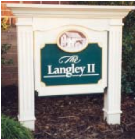
Vinyl lettering on 24-by-30-in. overlaid plywood panel. Graphic is vinyl, printed on the Gerber Edge®, mounted on PVC panel. Fluted 6-by-6-in. posts, the cap and crown are finished with Ronan enamels [T.J. Ronan Paint Corp., 800-247-6626, www.ronanpaints.com].
