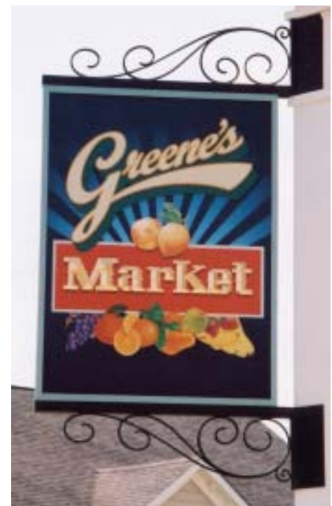
Greene's is cutout 1/4-in. Sintra PVC, finished with 1Shot enamel. Market is routed in 1-in. Sign-Foam high-density urethane board, finished with 23k gold leaf. Graphic is vinyl printed on the Gerber Edge®, applied to the 36-by-51-by-3/4-in. overlaid plywood panel, which is finished with enamel. Sign is mounted on wrought iron brackets.
