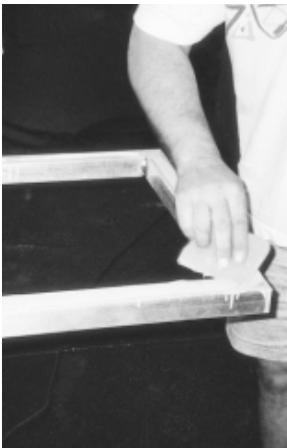
Spreading the adhesive
