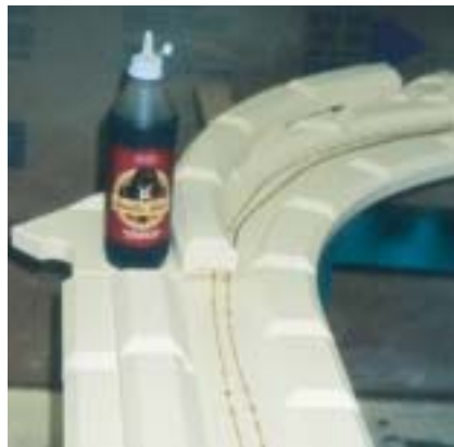
Figure 5. Applying the glue to the back-ground panel for the raised sections
