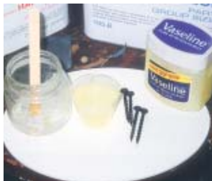
Figure 27. Screws, coated with Vaseline, were epoxied in place so they could be removed when the glue set.
