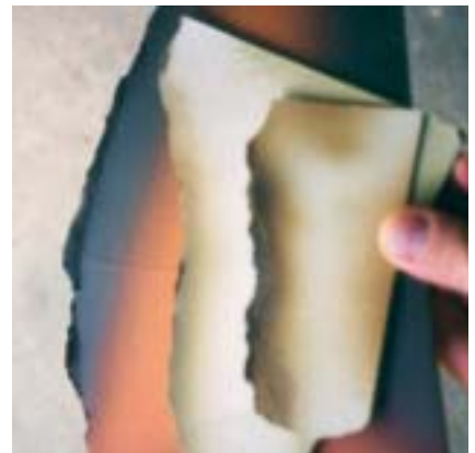
Figure 24. Note the torn edge on the spray shields
