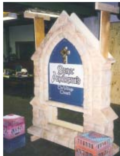
Figure 30. The panels glued into place
