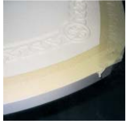
Figure 18. Before painting, the HDU was masked where glue would be applied
