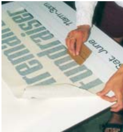
9. The bottom portion of the lettering is applied to the panel and squeegeed, creating a hinge for installation.
