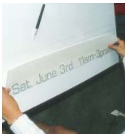
6. After matching centerlines, Darla positions the bottoms of letters on the guideline.
