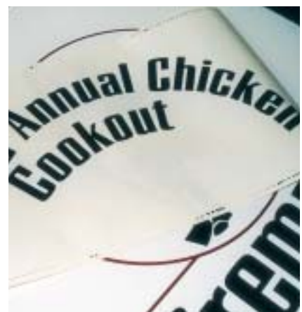
15. Note how the lettering was nested on vinyl to conserve material.
