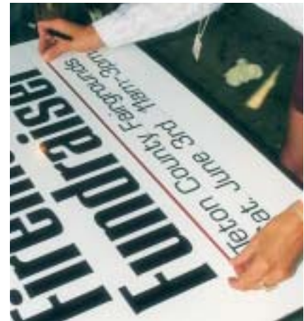
11. The stripes are applied by hand with no application tape, as are the outside borders.
