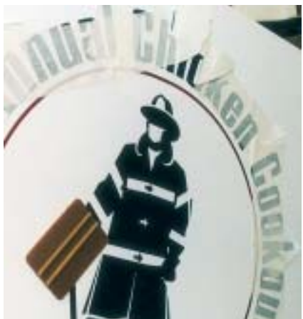
16. The first section of arced text was applied at the center of arc over the H, then the other section was applied.
