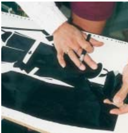
1. Weeding goes quickly, using the tip of the No. 11 X-acto to pick up the film where necessary.
