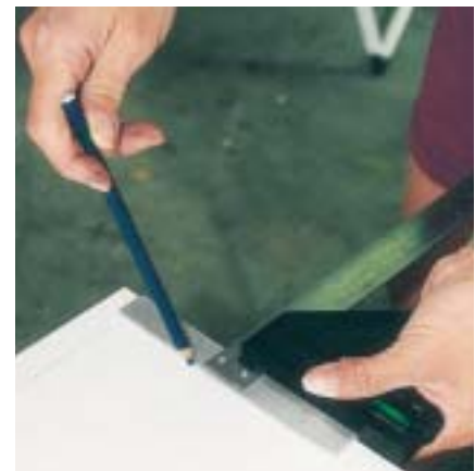
3. A picture framer's matting combination square is used to lay out corners and borders.
