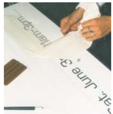
7. After application, the masking is peeled back at 45 degrees, flush with the surface.
