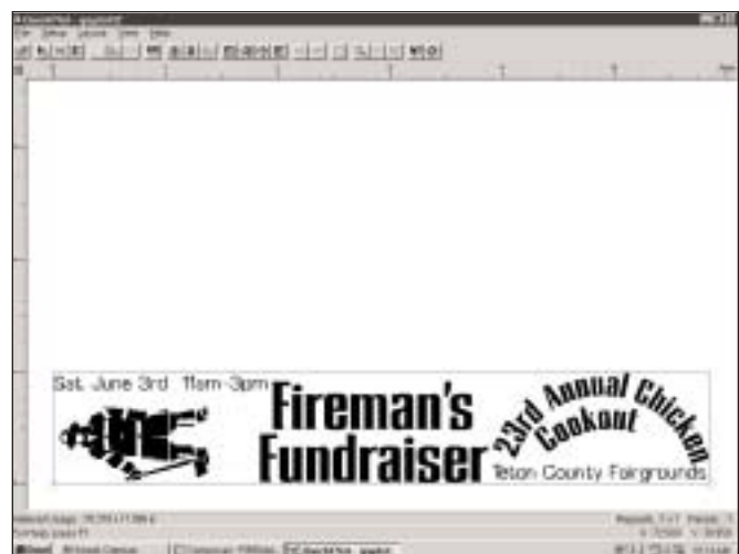
The lettering and graphics were "nested" in Composer to conserve vinyl before being sent to the plotter. Here are the black graphics ready to cut.
