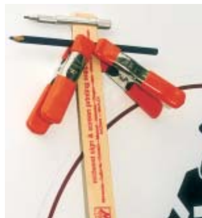
14. A modified yardstick compass carrying a Stabilo is used to mark the radius of arc using measurements from the design on the screen.
