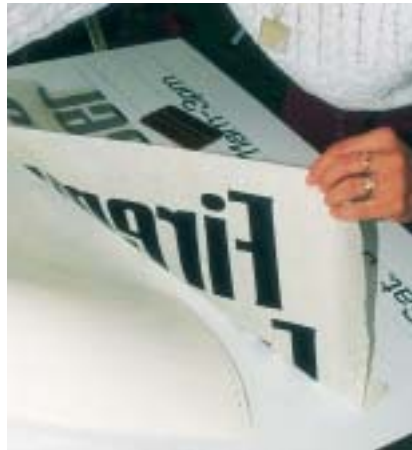
10. Next, the top section is lifted, the liner is removed, then the vinyl squeegeed.
