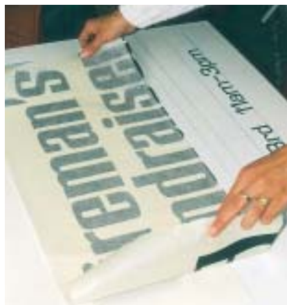
8. For larger graphics the vinyl is masked, lifted, then reapplied to the backing paper so the adhesive across the bottom 3 in. of the vinyl is exposed. This makes it easier to position during application. Note bottom guidelines already drawn on the panel.
