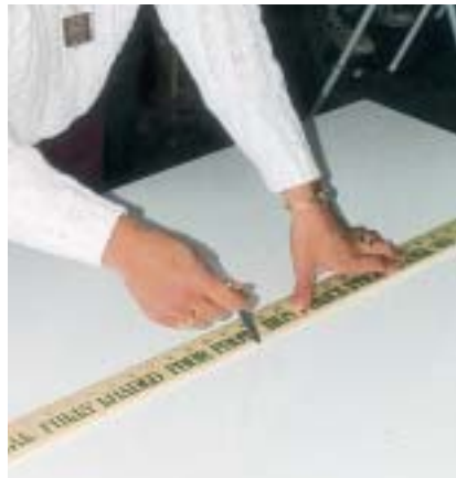
2. Centerlines on the panel and graphics speed application. Guidelines were drawn with a Stabilo pencil.
