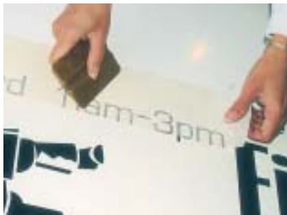
4. Transfer tape is applied to the vinyl, leaving the bottom \frac{1}{16} in. of the letters exposed.
