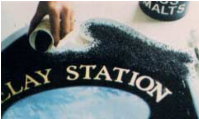
9. A generous layer of smalt, about 1/4-in thick, is applied to the wet binder.
