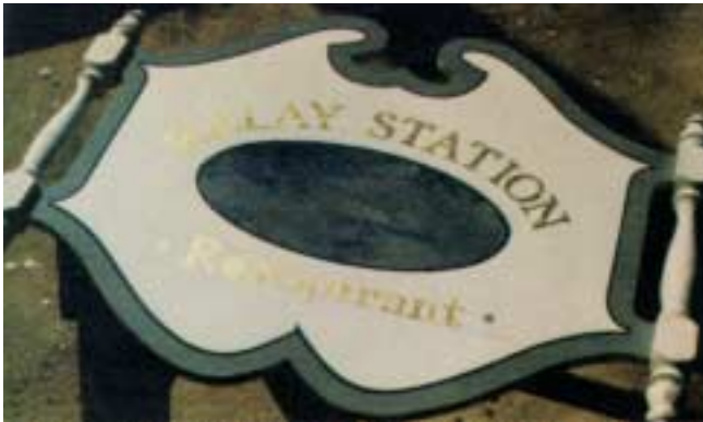
5. The lettering is gilded and burnished, and both panel and border are outlined.
