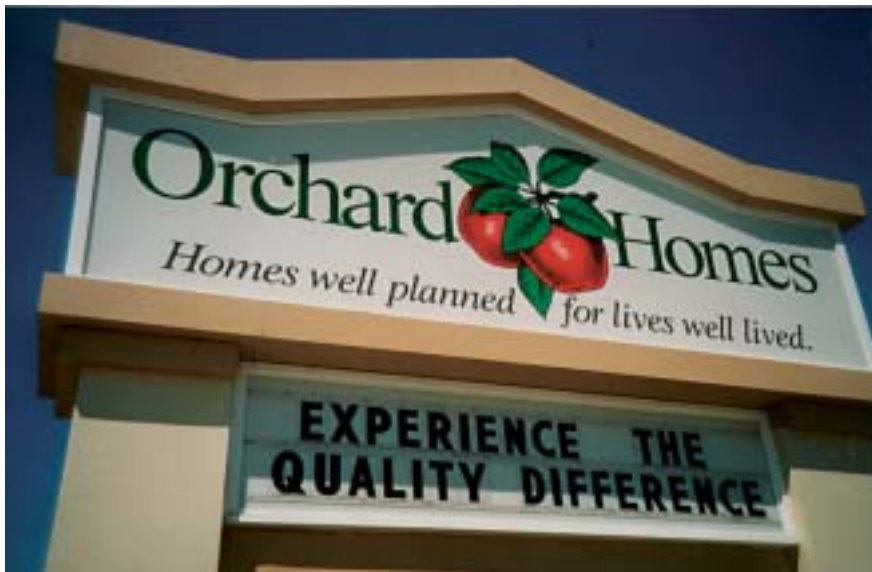
This is an unusual 2-line, 6-in.-character changeable copy sign application on a 12-by-16-ft. double-faced pylon sign. The sheet-metal cabinets and retainers are painted; the sheet-metal pole covers and embellishments have a texture paint finish. The graphics are 3M translucent film on white polycarbonate faces. Montana Signworks, Helena, Montana
