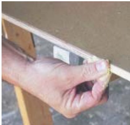
Figure 6. Using my fingers, I apply exterior carpenter's putty to all exposed edges. Since the edges have been rounded over with the router, this process goes quickly. At this point the edges are extremely smooth, so the danger of splinters is nil. In my left hand is a ball of putty ready to be inserted into the dispensing tool.
