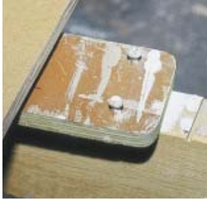
Figure 4. Since the screws are placed the width of a 2-by-4 they grip the sawhorse and keep the panel from sticking to the support due to paint running under the panel.
