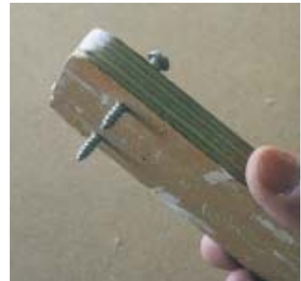
Figure 3. This handy block keeps the panel off the sawhorse and makes it easier to prepare the edges. It is made from scrap MDO and some screws. These can be placed between stacked panels if work space is limited.
