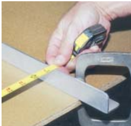
Figure 1. A piece of aluminum angle serves as a guide for the circular saw. It is held in place by clamps on each end. Since the distance from the blade to the edge of base plate is 1.5 inches, I place the straight edge at 37.5 inches.
