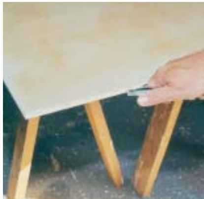
Figure 9. The dust is blown off with compressed air, with special attention given to the edges. The tops of the sawhorse are also cleaned so that there will be less chance for sawdust to migrate into the wet paint later. Usually several jobs are prepared at once with the floor being swept before the paint is uncorked. Fans in the shop are now turned off to help settle the dust.
