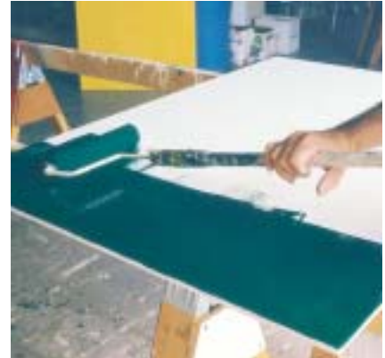
Figure 21. A deep green is mixed using Chromatic Bulletin Enamel. The process of rolling is repeated—long, parallel strokes with a heavily loaded roller.
