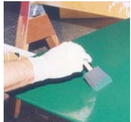
Figure 24. A foam brush is stroked lightly over the panel to pop the bubbles. I am not spreading paint, but just allowing the weight of the brush to smooth out the imperfections. Don't forget the edges. Drips are cleaned up with this step, too.
