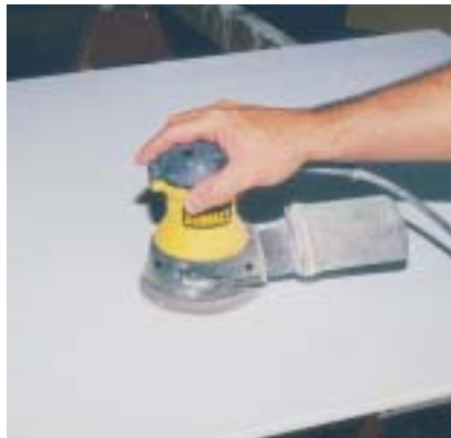
Figure 20. The following day the primer is sanded with a 120-grit disk. The edges are usually sanded by hand. A dust brush does a good job of removing most of the sanding debris. The panel is also quickly wiped down with a tack rag.
