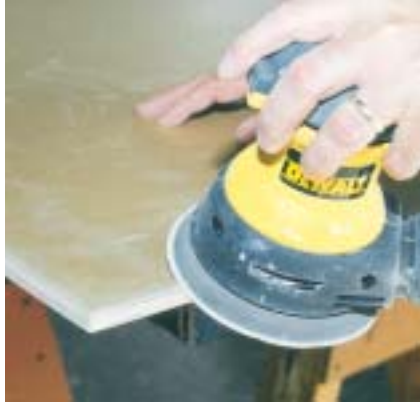
Figure 8. After the putty dries, the edges are sanded with 120-grit sandpaper on an orbital sander. You can also do this by using a folded piece of sandpaper in the palm of your hand. The paint will now have a continuous surface on which to adhere, without a “seam”.
