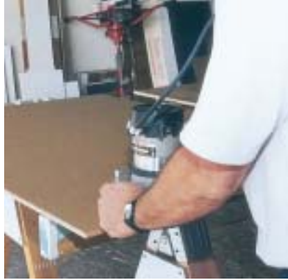
Figure 5. A 1/4-in. rounding-over bit is placed in a router. The edges of the panel are routed (both sides) to form a smooth, rounded edge. Most paint failures occur where the paint film must try to wrap a sharp angle, thus the sharp points are removed. I keep this bit in one router all the time. It is a simple procedure to just pick it up and go to work without having to readjust with each use. Other routers are equipped with other often-used bits.
