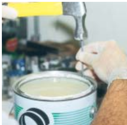
Figure 12. Before a new can of paint is used, holes are driven into the lid channel to keep the paint from building up and preventing the lid from seating properly. Since I am dealing with solvent-based paints I normally try to wear latex gloves to protect my skin. The paint is stirred to get the heavy deposits off the bottom of the can.
