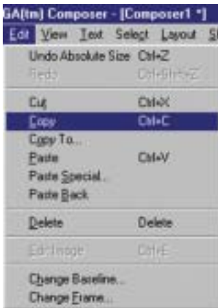
Here's a typical Edit pull-down menu. This one is from the Graphix Advantage Composer in Gerber's Omega software. Note the shortcut keys beside many of the commands. The optional shortcut keys you can use while in the pull-down are underscored.
