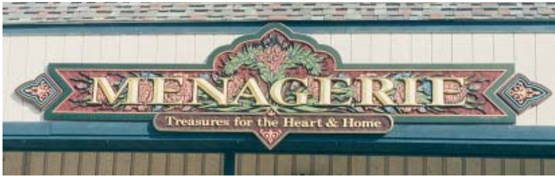
3-by-16-ft. high-density urethane sign, with carved, gilded letters applied to the sandblasted background. Graphics and background have an acrylic latex finish.
