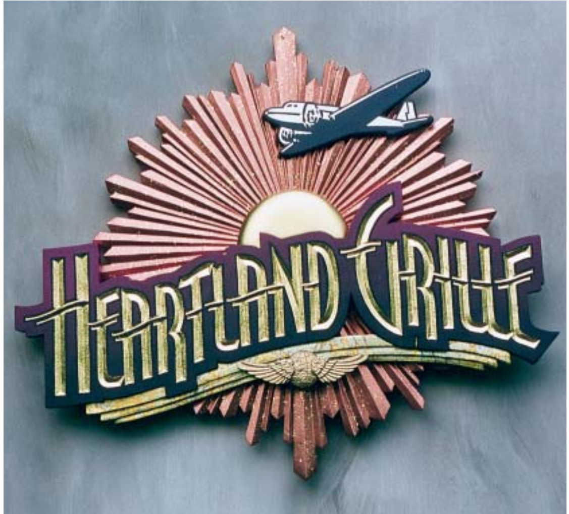
3-by-3-ft. high-density urethane sign, with acrylic latex finish on lettering area and hand-carved, gold-leafed letters. The carved prismatic sunburst has a sprayed copper finish, sprinkled with gold glitter. Wings are carved with bronze spray finish.
