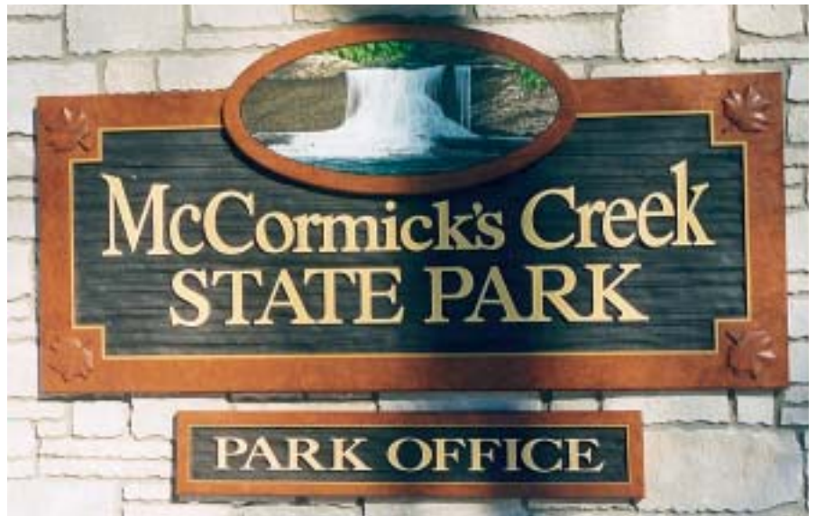
4-by-8-ft. high-density urethane sign, sandblasted with acrylic latex lettering, background and pictorial. Border has acrylic glaze and carved leaves.
