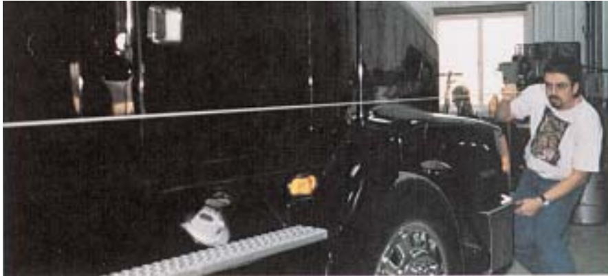
Figure 1. Start by laying a level line of tape down the side of the truck.
