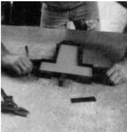
Figure 10. When wrapping the letter, use just a few magnets to hold the trim in place. The fewer magnets you use, the less work. It's faster, too. Once the trim is fitted, press several magnets against the trim to ensure a close fit.
