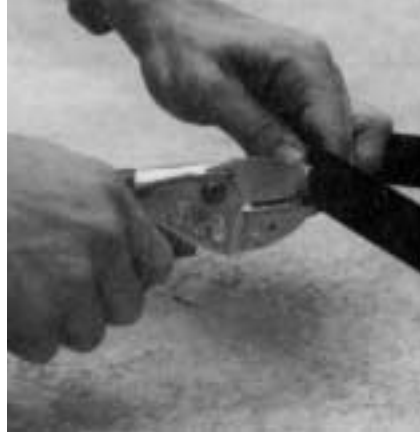
Figure 8. Remove the trim and make the notch. Caution: When cutting the notch with a notcher do not cut too deep. You don't need to remove the entire bevel of the trim to get enough space to allow a sharp crease. Removing about half should be enough. If there's a gap in the crease of the trim, you removed too much. Experiment with a scrap to get the correct notch. This step will be repeated several times on common letters, such as E or T, so it won't take long to get the hang of it.
