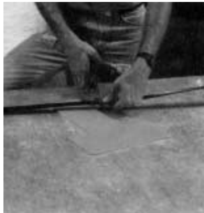
Figure 5. Cut the letter trim to length with the tin snips. We buy it in 10-ft. strips or in 100-ft. rolls. Precutting the trim into a smaller size, of course, makes it easier to work with.
