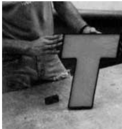
Figure 16. Finally, wipe the face clean, and give the trim a final inspection to make sure it is seated against the face of the letter and bonded to the plastic. If everything is okay, your letter is complete and it's time to get started on the next one. With practice you'll find that the process goes quickly and smoothly.
