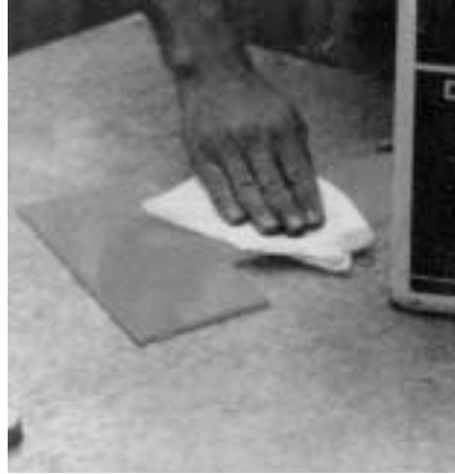
Figure 2. Clean the back of the letter with denatured alcohol. The alcohol dries quickly, removes dirt and oils, and doesn't leave a residue. Thus, the trim will fuse better to the plastic.
