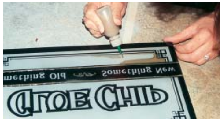
Figure 6. Use a small squirt bottle to apply the glue to the frosted areas that will be chipped.
