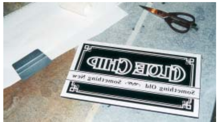
Figure 2. Apply the mask over the dry asphaltum.
