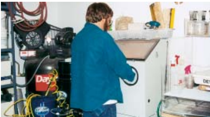
Figure 3. Mike blasts small glass pieces in a blasting cabinet.
