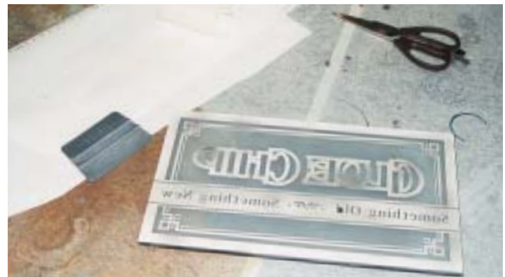
Figure 4. Lightly sandblast the exposed areas.
