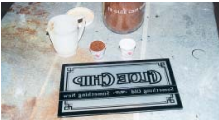
Figure 5. Masking removed and glue ready to mix
