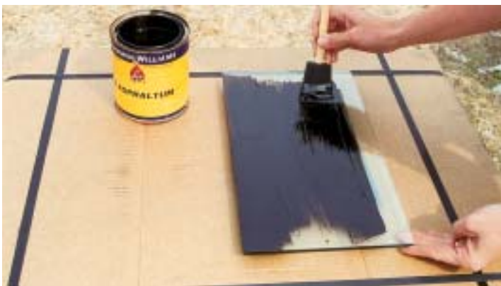
Figure 1. Apply the asphaltum evenly.
