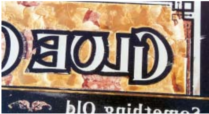
Figure 9. The glue pulls the glass off in small chunks.
