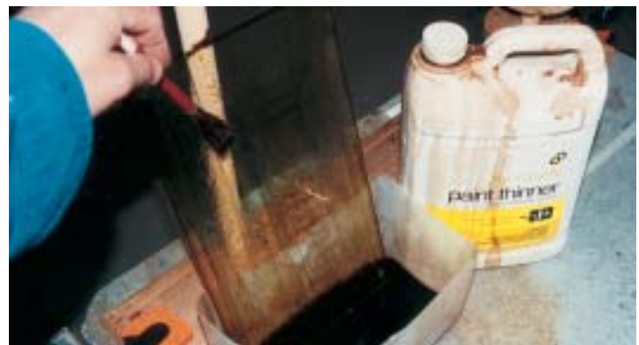
Figure 12. Flood the thinner over the glass with a small camel-hair brush.
