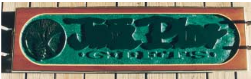
Figure 6. After enamel painting was done, the sign was ready to gild.
