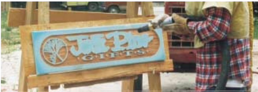
Figure 3. Sandblasting took about five minutes per side.
