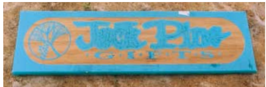
Figure 2. The panel, with stencil cut and ready to blast
