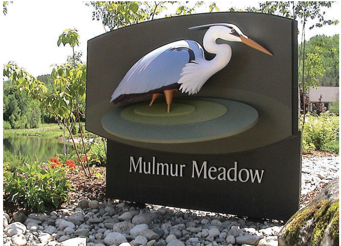
Standoff-mounted aluminum flat-cut letters on 5-by-5-ft. high-density urethane board. The upper metal frame is concave and the bottom panel is pebble textured. The rings representing the water are mounted on standoffs at an angle. The heron is approximately 45 in. long and up to 10 in. thick.
