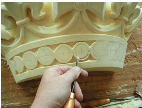
17. Here I'm detailing the last part of the crown. After this was complete, and the crown had been applied to the sign, I carved and added the sphere and cross at the top.
