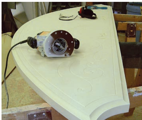
4. I finish up the scrollwork , and then rout the edge cove.
