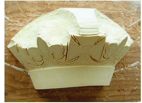
12. Once all the angles are right, I screw the carving to a sheet of plywood from behind and transfer the image to the block. Then using my Dremel and a straight bit, I just start working my way back.
