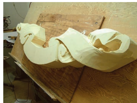
6. When I begin rough-carving the banner, I use the highest point for reference and work back to the lowest point.
