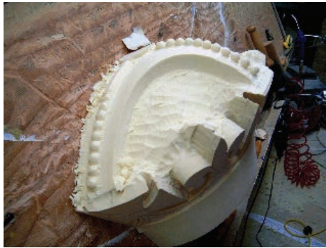
13. I use gouge and an assortment of hand files to rough in the beads that run along the top of the crown.
