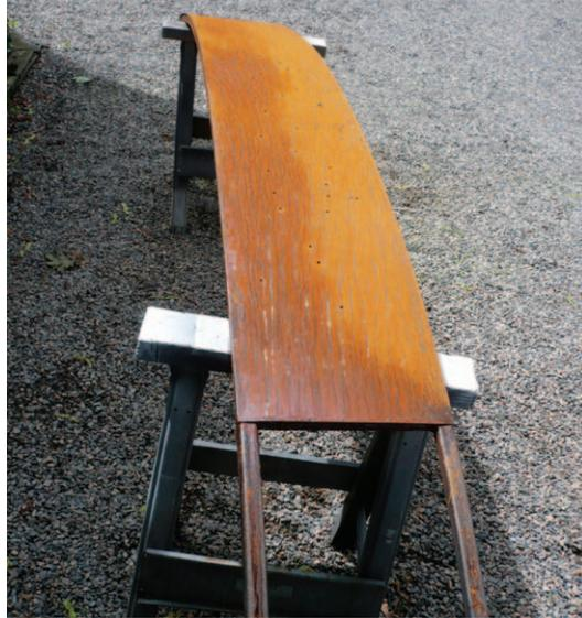
**3. Rust the panel: 2 hours** Table salt dissolved in water was used to expedite the rusting of the steel. Once the effect was right, I neutralized it with a solution of baking soda and water.
