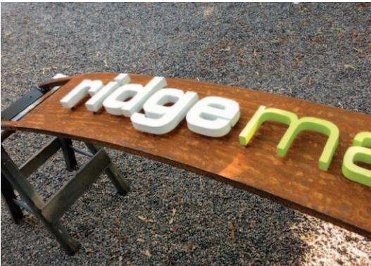
**4. Cut, paint and mount letters: 6 hours** The letters were cut from PVC board on the CNC router, finished, then mounted on standoffs.
