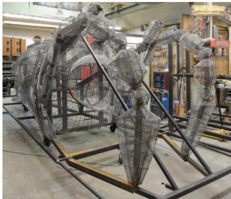
**The more complex the shape, the** more difficult it is to shape and tie on the galvanized mesh. While that may be true, it's also true that the more complex the shape, the more interesting the final result will be. Once the wire is all secure it is time to begin sculpting the final shape.
