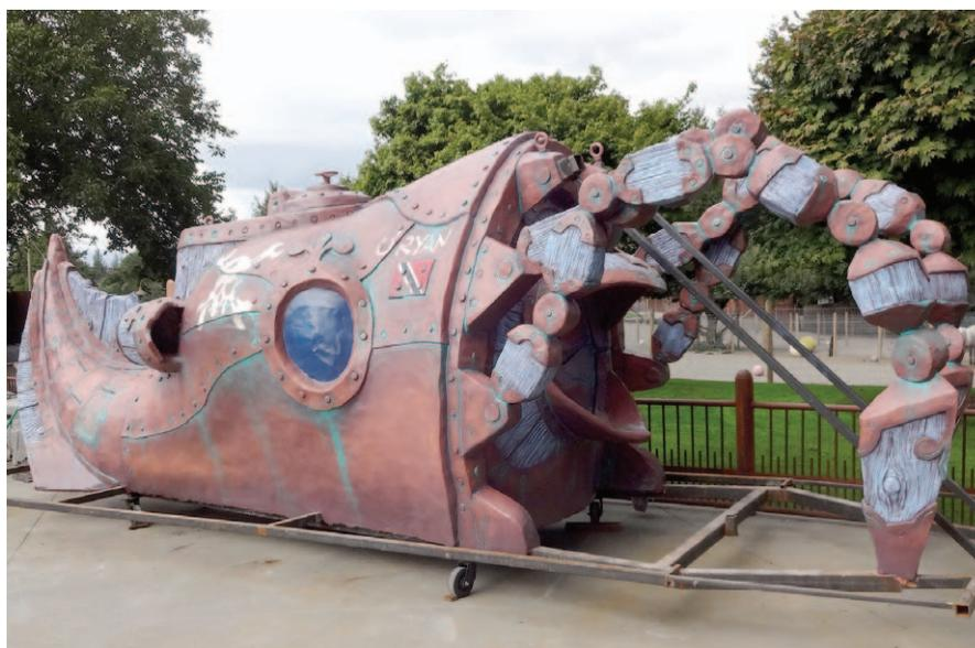
The final paint job was a pleasing combination of warm and cool colors. Once painted, it was pushed out of the shop to make room for many more pieces yet to be done. It will be placed on a concrete footing on site and then the deck will be poured around it, burying the remnants of the shipping frame.
