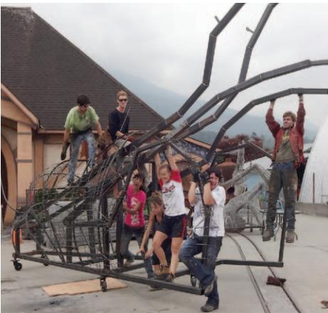
**The eager crew tests the** heavy, welded steel frame for the Kraken. Each piece was built on removable wheels so we could move the pieces around the shop and yard. Lift points were also designed from the start.
