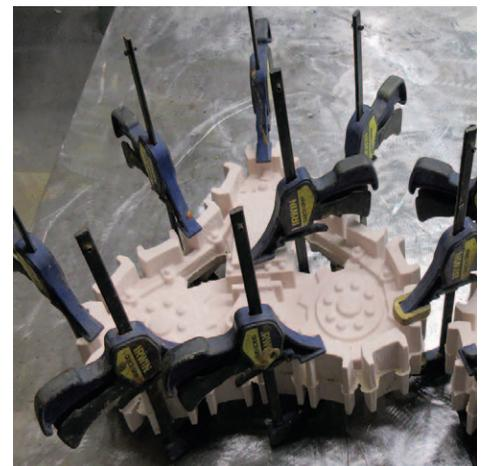
They were done half at a time to be glued back to back. The inside pieces had rectangular blocks to allow them to be glued to the chassis. Once the pieces were assembled, they were cleaned up a little with a handheld die grinder.
