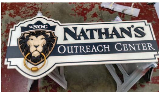
**Assemble and complete the sign: 75 minutes** Once the components were cut and finished, we mounted the letters on the panel using VHB tape. I hand lettered the secondary copy with Nova acrylic paint.
