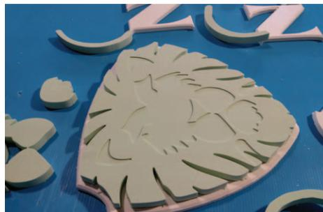
I did the same thing on the mane layer, routing an inset to accept the face components, which were also cut from 1-in. HDU.
