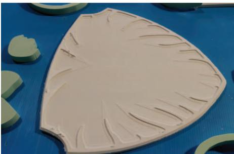
**Router-cut components: 1 hour** The letter components for the lion's head were cut to shape on a CNC router. The letters were cut from 1/2-in. Sintra PVC board [www.graphicdisplayusa.com]. For the lion's head, I started with a backer of 1/2-in. Sintra PVC board to give me the rigidity I wanted. I routed an inset to accept the next layer, the mane, which was 1-in. Precision Board HDU board [www.precisionboard.com].
