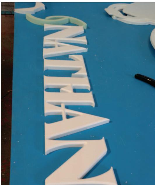
**Finish letters and panel: 90 minutes** The letters were finished with Nova acrylic paint. The sign panel was cut from a 4-by-8-ft. sheet of 3/4-in. Sintra PVC board then finished with Sherwin Williams Superpaint. We taped off and painted the panel and border with Nova acrylic paint.
