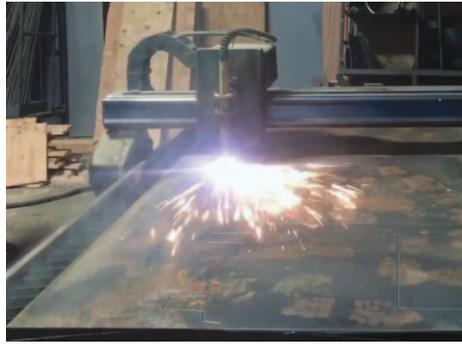
We cut the flat steel pieces on our MultiCam CNC plasma cutter. With CNC, everything fits perfectly. I never even had to use a level or square to assemble them.
