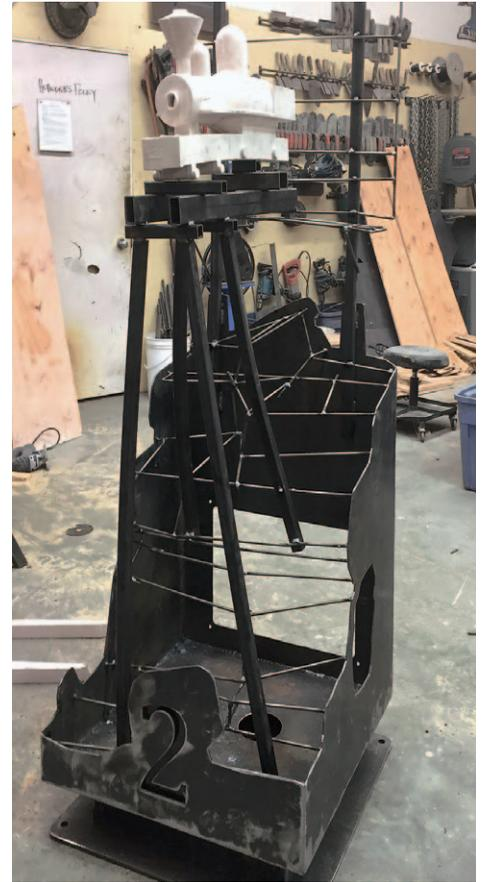
A pencil rod frame was welded to the basic structure to form the bones. Expanded lath was tied to this framework to hold the sculpting epoxy skin.
