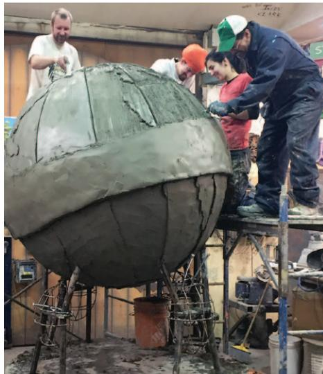
We then troweled on a thick coat of fiberglass-reinforced concrete. Once it had set the perfect amount our crew carved in the detail. The globe was to look like it was made from thick, curved planks of wood. The lettering on the band was hand carved in. To speed things up, I laid it out in sections, using an overhead projector and transparencies.
