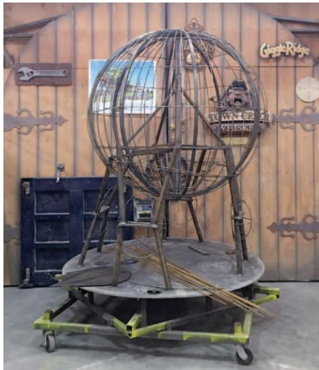
The structural steel supports for the globe are cleverly hidden in the arms and legs of the lower bugs. A final substructure of ¼-in. round steel (pencil rod) forms the armature to which we will attach the galvanized steel mesh.
