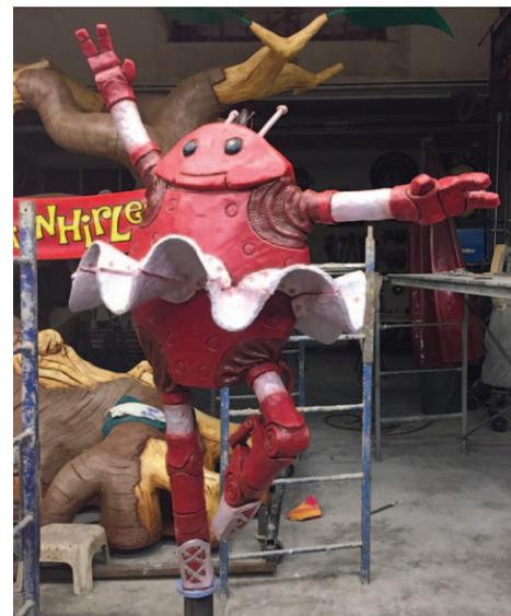
The ballet dancer, who is to be perched on top of the globe, has a sturdy, welded steel frame running through it. The main body is sculpted from fiberglass-reinforced concrete while the arms, legs and tutu are sculpted from Abracadabra Sculpting Epoxy. It is hand painted with three coats of Sherwin-Williams house paint and then glazed to bring out the textures and add character.
