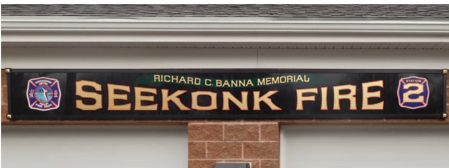
22K gold leaf Florentine Realgold film letters over high performance vinyl film on 21-in.-by-16-ft. black aluminum composite panel with aluminum J-mold trim and OVC corners. The department logo and station number are digital prints.
