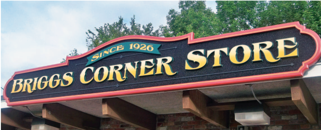
CNC-routed 32-in.-by-16-ft. panel of 2-in. HDU sign finished with Matthews Satin and black smalts, with an airbrushed blend on the main copy. The font is Esoteric from LetterheadFonts.com.
