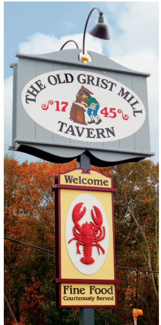
Hand-painted 67-by-84-in. sign on 3/4-in. overlaid plywood sign with mahogany trim, finished with matte acrylic latex paint. The center art and lettering was hand painted with enamels. The Welcome panel uses 1/4-in. aluminum composite letters on a 1-in. PVC panel, finished with Matthews acrylic polyurethane paint. The lobster is a VectorArt 3D clip art image [www.vectorart3d.com], CNC-carved from HDU board, with details added by hand.
