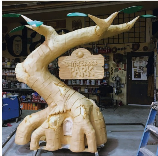
After the three coats of base color had dried it was time to begin the glazes. As always we started with the lightest glaze. It was brushed on and wiped off carefully. The glaze left in the texture and cracks made these details jump into view.
