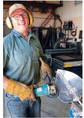
The leaf shapes were cut from 10 gauge steel plate, bent to shape and then welded to the half-inch steel rod that forms the stem. A little grinding makes everything nice and smooth. Once we were done they were sent out to the powder coaters for the green color.
